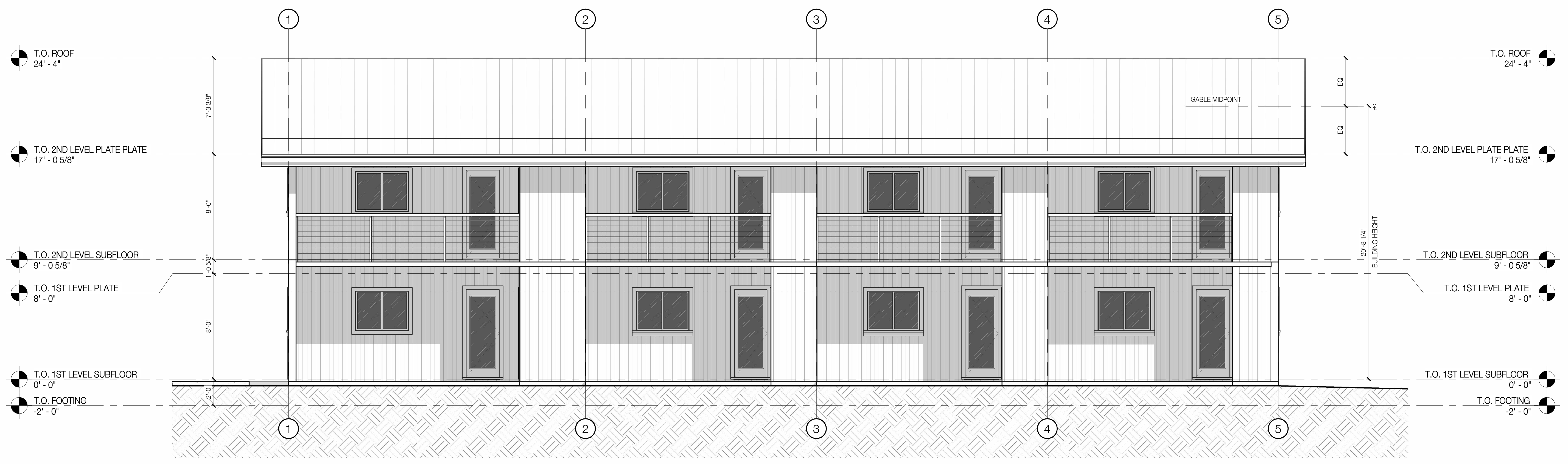
1 NORTH BUILDING ELEVATION 1/4" = 1'-0"
